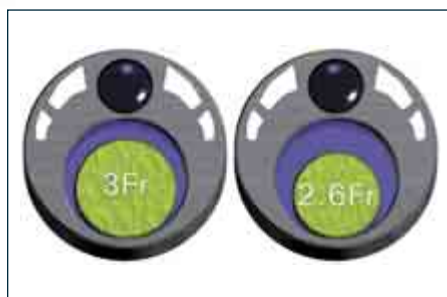
2.6Fr sheath diameter offers 56.4% more irrigating capacity than a 3.0Fr sheath.
